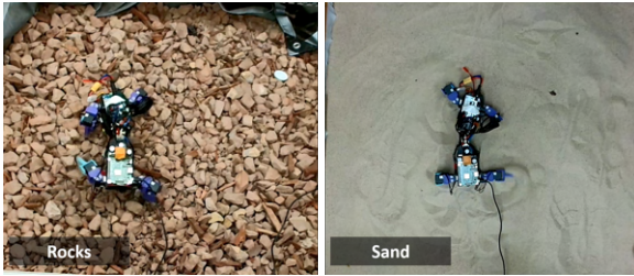
Fig. 8. Qualitative evaluation of the robot on uneven terrain. The hybrid Hildebrand+RL strategy enabled successful traversal on (left) rocks (sizes between 2-4 cm) and (right) dry sand.
