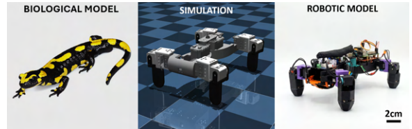
Fig. 1. Biological and robotic model. (left) The fire salamander ( Salamandra salamandra ) is a common species of salamander found in Europe. (middle) The robot model in the Mujoco simulation world. (right) 3D printed robotic salamander.
