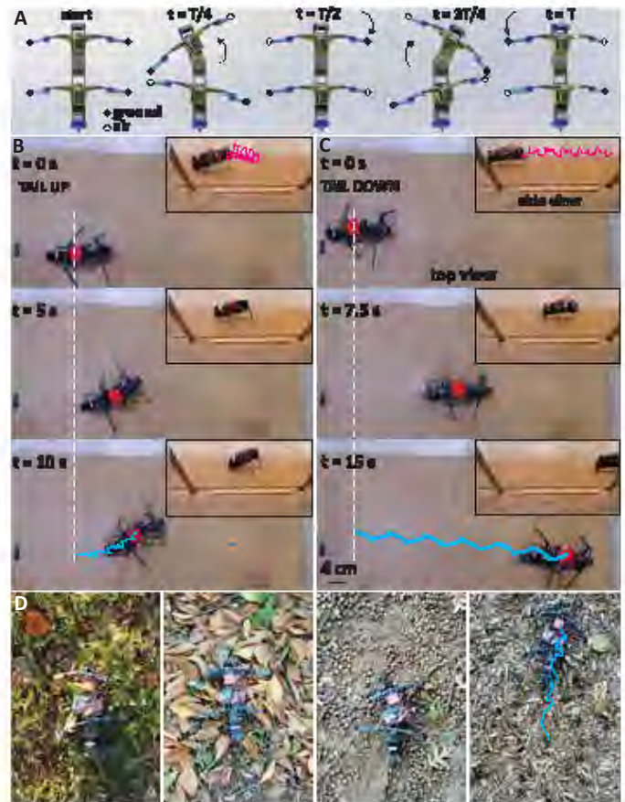
Fig. 3. The importance of passive tail use on forward locomotion of individual robots using a diagonal gait. (A) Leg states (white, in air; black, on ground) and joint angles for a diagonal gait. T represents the gait cycle. All the robots use diagonal gait during the forward and backward locomotion. (B) Forward locomotion on a flat surface (particle board) with the passive tail in the air. Blue trajectory shows the CoM trajectory during walking ( n = 4 cycles). Insets show the side view of the robot and the tip trajectory (pink). (C) Forward locomotion on a flat surface (particle board) with the passive tail on the ground. Blue trajectory shows the CoM trajectory during walking ( n = 6 cycles). White dashed lines show the starting position, and insets show the side view and tip trajectory (pink) of the robot. (D) Tail down quadruped walking on natural terrain (grass, acorns, leaves, and mulch; movie S2). An example tail trajectory (blue, six cycles) of the robot is given in the last image.
